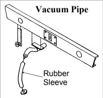
Fit the vacuum pipe castings. Solder the top of pipe and hose support (known as the dummy) casting to the buffer beam. Push the end of pipe coupling casting into the rubber sleeve and then push the sleeve onto the top of pipe casting. You can then leave the pipe hanging down (this was the case in some photos I looked at ) or you can secure the end of the pipe to the dummy with a spot of low melt solder so that it is secured as required by good railway practice. There are also castings for
