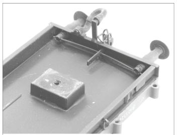
Bogie mounting box and also note the position of solebars in relation to buffer beam
